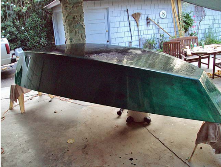
Pic 5 Here is a pic of the hull nearly completed, less its bottom coat of graphite infused epoxy and marine grade paint. Note, no more bailing wire; it was removed in the filleting process. Seams are nice and clean.
