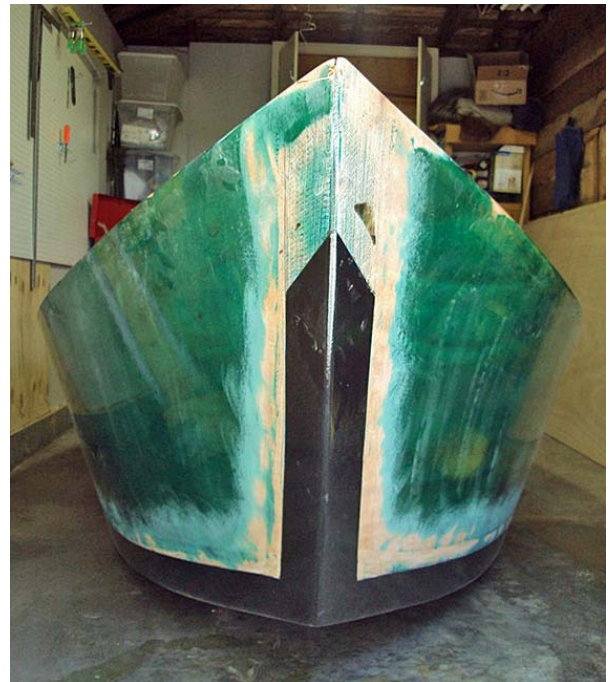
Pic 5 Here is a pic of the hull nearly completed, less its bottom coat of graphite infused epoxy and marine grade paint. Note, no more bailing wire; it was removed in the filleting process. Seams are nice and clean.
