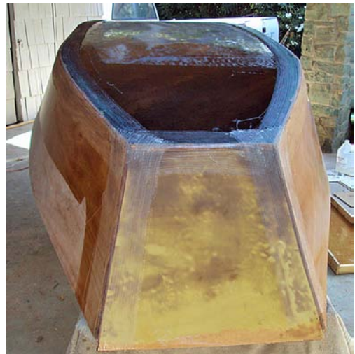
Pic 4 Now the hull comes together, addition of some 12 oz biaxial tape and refining of the chimes. She is starting to take shape. With some sanding you won't notice the seams at all.
