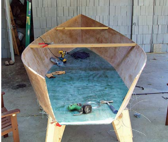
Pic 3 In this photo you can clearly see the baling wire holding the panels together. True stitch and glue construction.
